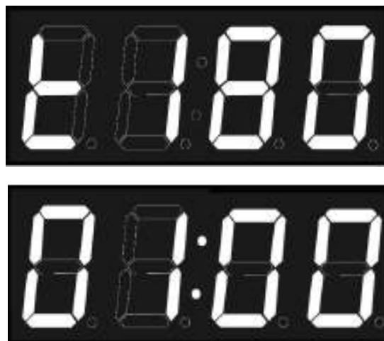
Figure 12. Example. Cooking 180°C for 1 minute
