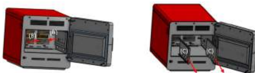
Figure 21. Removal of screws and side plates
